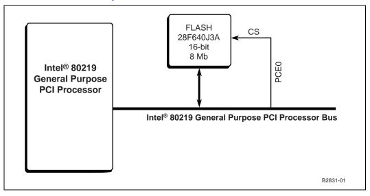
Under normal operation, the very first instruction access by the Intel XScale<sup>®</sup> core begins at location 0x0 on the 80219 Internal Bus. By default, address 0x0 is pointing to PCE0 where flash is located.
